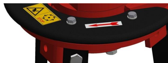
Figure 25 Direction of rotation Rotary Cultivator
