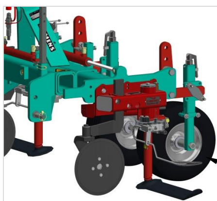
Figure 5 Support wheels for height guidance
