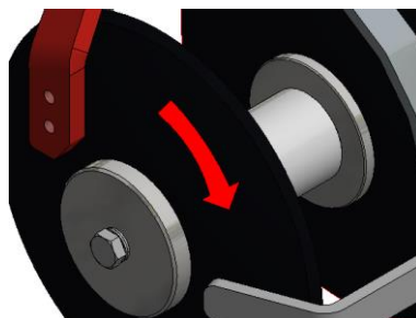
Figure 20 Direction of rotation of the disks
